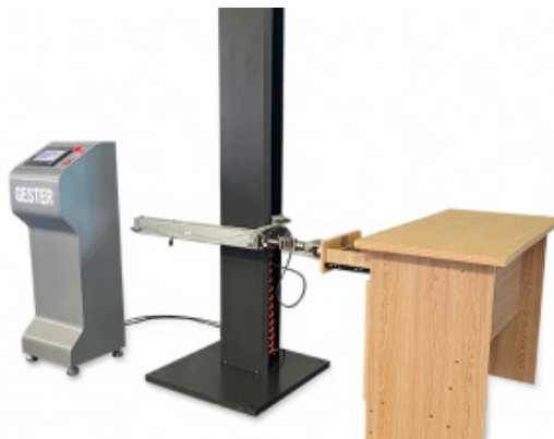
Fig. 8.1.3: Testing drawer joint strength with pressure
