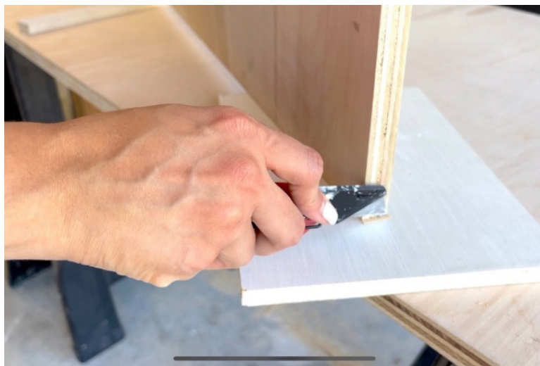
Fig. 8.1.2: Inspecting edge banding and finish
